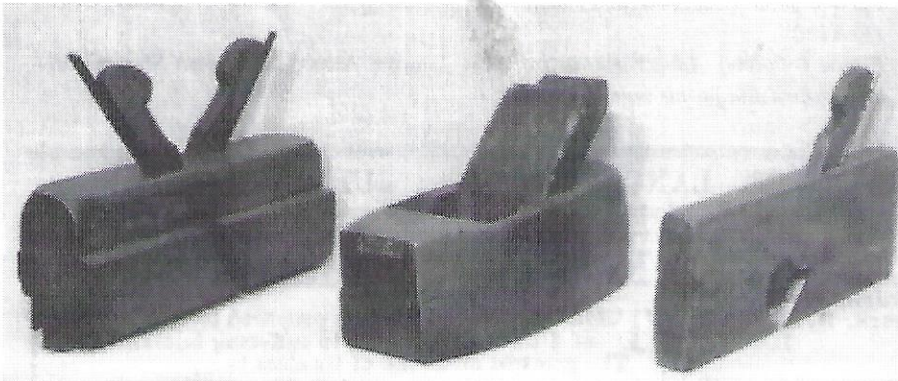
Figure 9. Illustrated are (left) a double tongue and groove plane (imprint E, length 8\frac{3}{8} inches), (center) a smoother (Imprint b, length 8 inches), and (right) a molding plane (Imprint d) length 9\frac{1}{2} inches.
