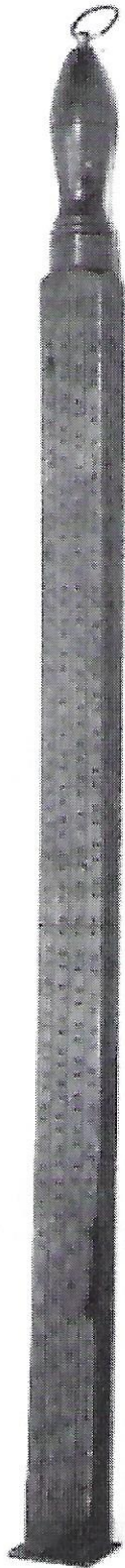
Figure 16. A unique lumber scale, 50 inches long with 16 hand-stamped scales ranging from 18 to 48 feet. The scale is marked with Imprint e (Richard Cammauf Collection).
